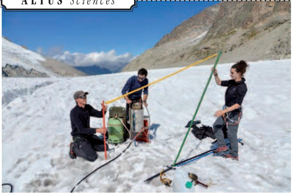
➤➤➤ years' probes. The GPS measures their movement and thereby the glacial flow, while the coloured part of the protruding probes indicates the loss in height.
